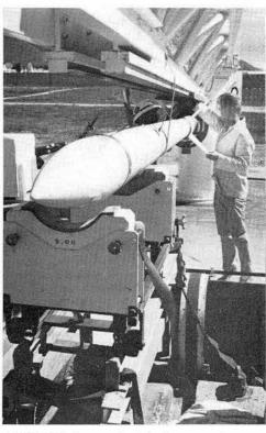
PAYLOAD is mated with the second stage and Nike booster on the rocket launcher by Jim Strascina (in helmet) and Bruce Barth.
